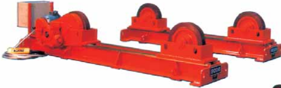
2/CR.200 Capacity 10 tonnes Vessel diameters: 600 – 3000 mm Weld speed: 75 – 1500 mm/min.
