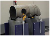
The ProCutter is equipped with adjustable pipe supports to level he pipe at cut location. Furthermore, the ProCutter can be equipped with a rollerball gutter that provides permanent horizontal support.
