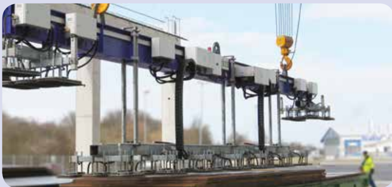
Heavy duty unit with carrying capacity of 32,000 kg
