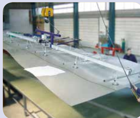
Handling of thin, special-format metal sheets
