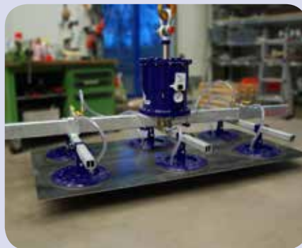
BASIC-LIFT with carrying capacity of 600 kg (BL 600/6L)
