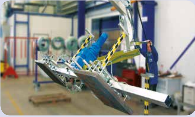
Turning lifter for heavy loads (over 1,000 kg)
