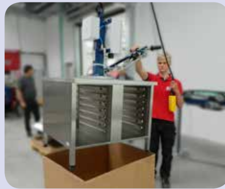
Handling of sheet metal cabinet with battery-powered unit
