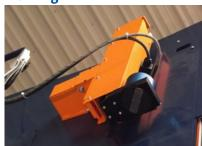
Optionally, a marking system can even further improve your productivity. The MPC can be equipped with punch, ink-jet or plasma marking systems.
