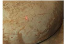
Laser triangulation measurement of the surface enables adaptation of the theoretical 3D cutting path to the deviations of the raw material.
