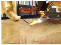
Cut radial and hill-side holes with weld preparations such as V and K bevels.
