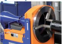
The self centring three jaw chuck is one of the factors influencing accuracy. It achieves high accuracy by clamping pipes securely, avoiding slip and creep (longitudinal movement) during rotation.
