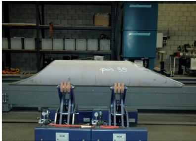
The SPC is equipped with adjustable pipe supports to level the pipe at cut location. These hydraulic pipe supports have coated wheels and a scissor mechanism to enable handling bow shaped pipes.
