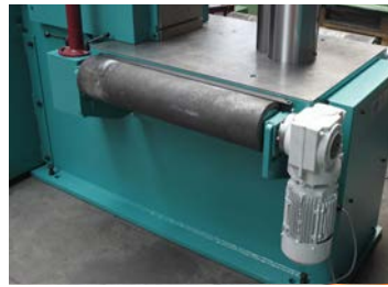
116 Driven roller directly at the machine
