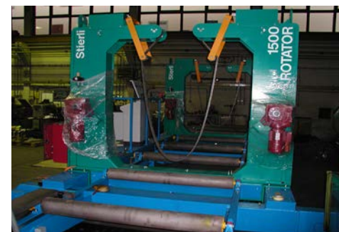
315 ROTATOR integrated in a roller conveyor (e.g beam welding line)
