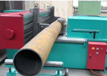
111 Pipe bending up to \varnothing 400\text{mm}
