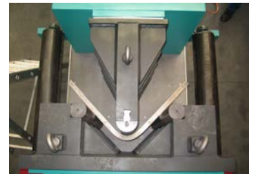
127 Bending of thick sheet metal
