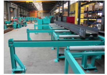
117 Cross conveyor system
