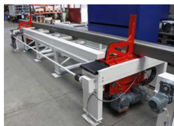
130 Turning device can be combined with roller conveyor
