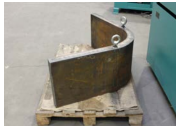
126 Heavy bending works e.q 400x60 mm
