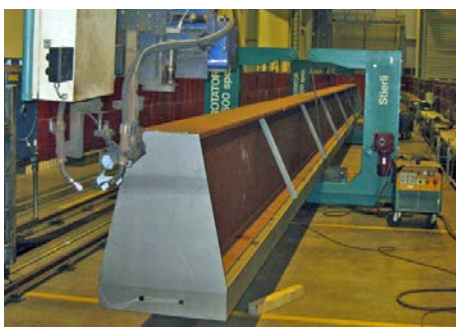
316 ROTATOR in combination with welding robot
