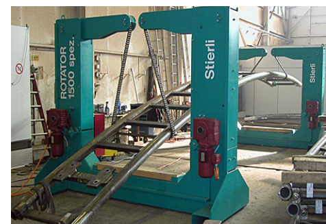
318 Durable chain for safety when turning
