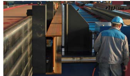
107 Beam straightening or bending in upright position
