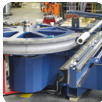
Radii of up to 1,500 mm with a precisely machined segment tool
