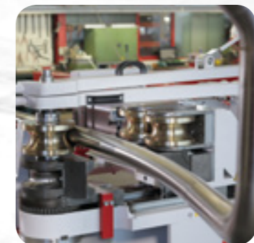
Free-form function for bending of large radii independently of the tool
