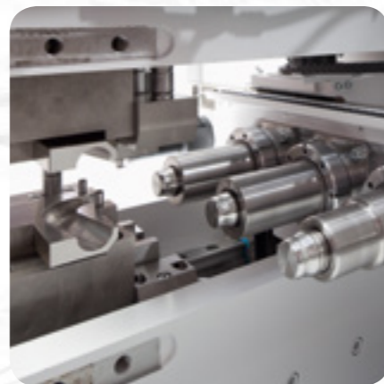
Fast and flexible in use: Forming tools on an axial tube forming machine
